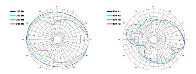
Fig. 8: Horizontally configured PD5322 - modeled vertical polar response
