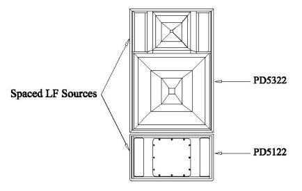
The PD5122 is simply the LF section of a PD5322. The similarity insures that the response of the LF sections will be identical. The acoustical crossover between the low and mid-frequency sections is 250 Hz. In the vertical polar plots (Fig. 3), note how well pattern control is maintained through the system crossover.
