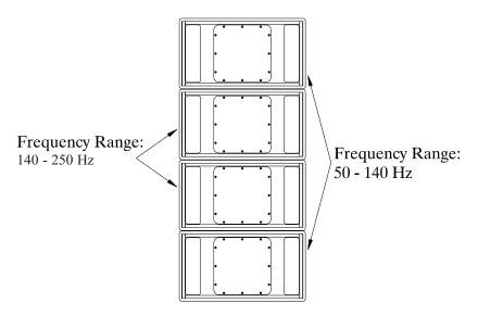
Fig. 9: Four-element PD5122 shaded array
