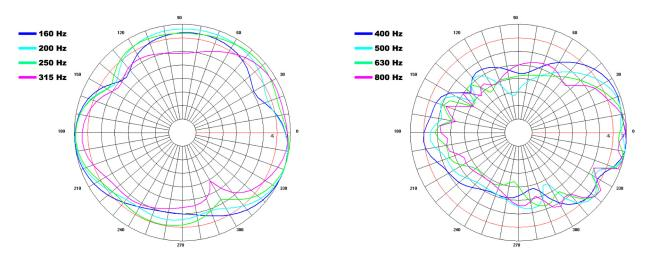
Fig. 6: Vertically configured PD5322 - modeled vertical polar response
