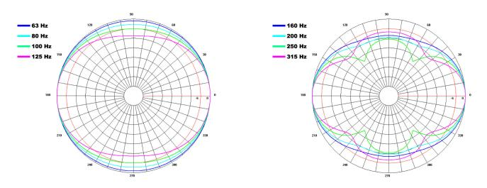
Fig. 10: PD5122 shaded array - modeled vertical polar response
